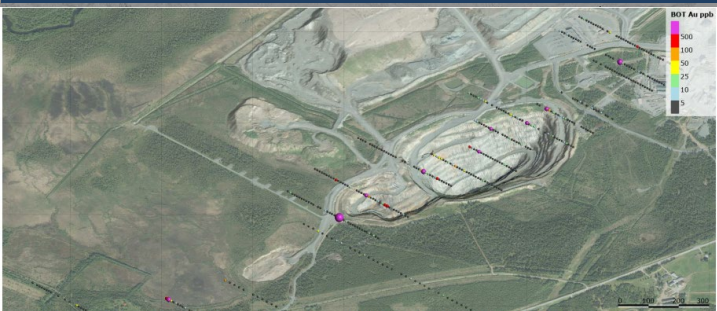
Isometric view of original BOT sampling results at Kittilä (BOT data from GTK's website).
